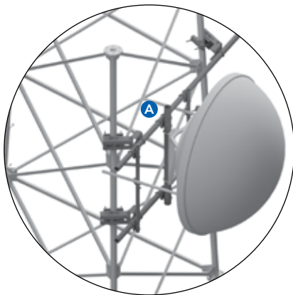
6' dish shown on 9' face tower using FMDS3-168 series mount
